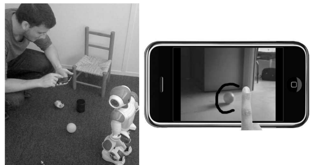
Fig. 1. Encircling an object allows the user to notify the robot that he wants to teach a name for this object and also provides an useful rough segmentation.
