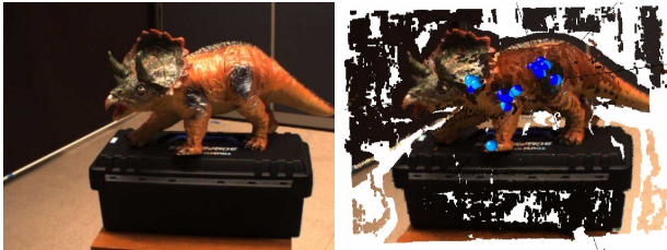
Fig. 8. Left : The left eye’s image of figure 7’s scenery. Right : The pose of the object is successfully determined using Rigid Motion minimization.
