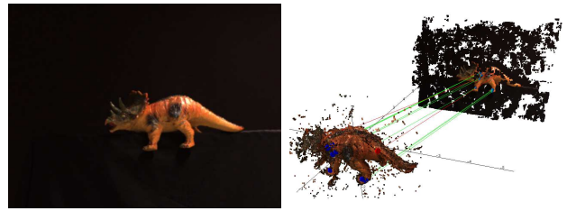
Fig. 9. Pose estimation on a uniform background is performed successfully at 1,7m with no occlusion.
