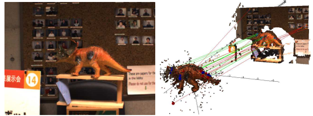
Fig. 10. Pose estimation under severe clutter is performed successfully at 1,6m with no occlusion.
