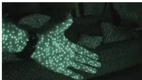
Figure 2: Semi-random laser pattern projected by the Microsoft Kinect. Photograph by J. Flatley, from his Engadget article .
