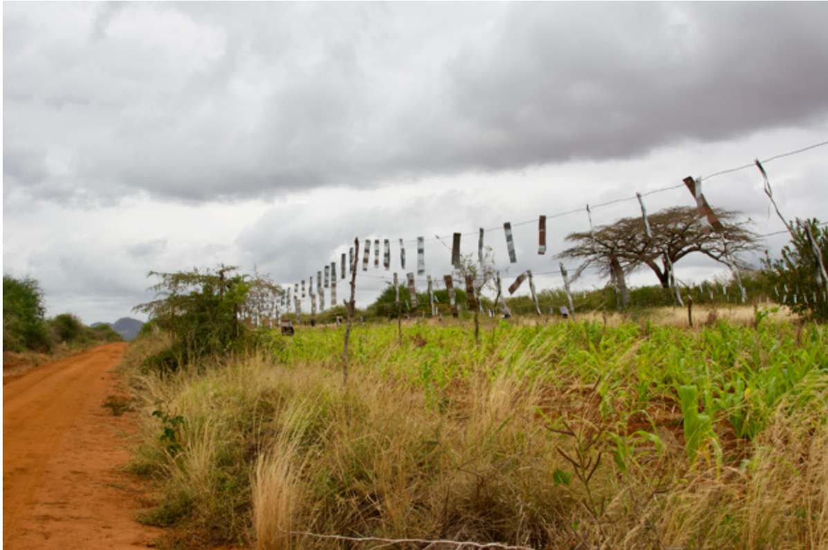
Figure 6. Kasaine double metal strip fence built and erected in experimental block 2 during trial 8 in the farming community of Sasenyi, Kenya. Photo taken by Sophia Corde.
