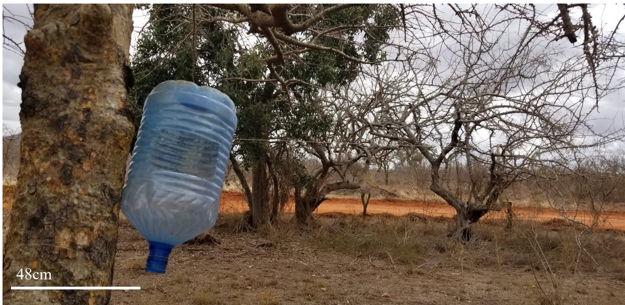
Figure 1. Aeolian harp created by using 40 lb test fishing line and a recycled 10L water bottle tested in Kivuli Camp, Kenya. Photo taken by Sophia Corde.
