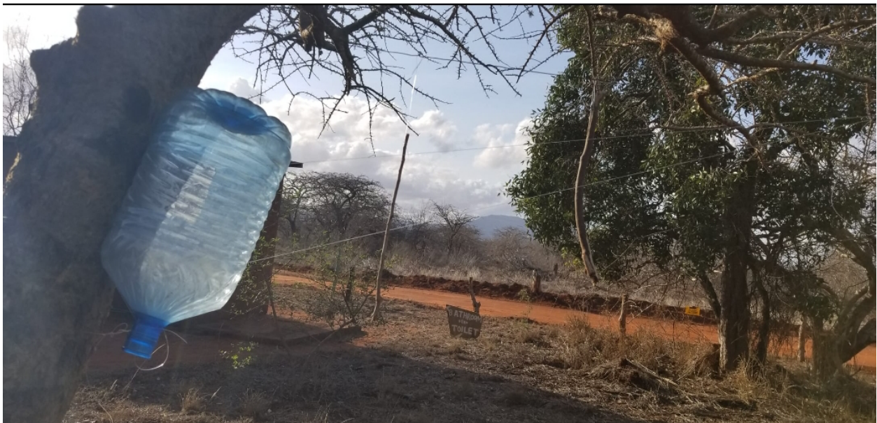
Figure 1. Pressure activated drum created by using 40 lb test fishing line, a recycled 10L water bottle, and sticks, tested in Kivuli Camp, Kenya. Photo taken by Sophia Corde.
