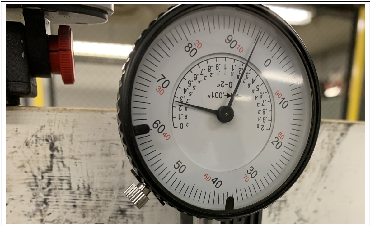
Figure 5.2: Final image of FeatureCAM's program's Z-axis test returning to its zeroed position for a value of -0.005".
