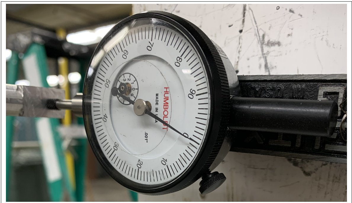
Figure 5.3: Twelfth image of RoboDK's program's X-axis test traveling to 0.5" for a value of 0".
