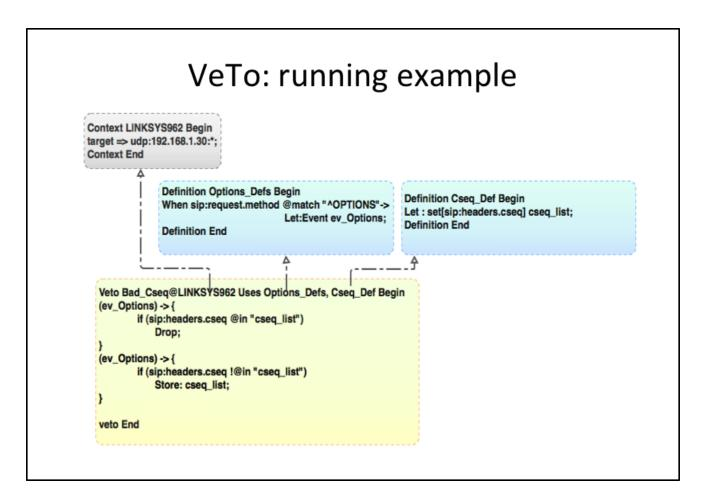
In this tiny slide, we present an example of a VeTo specification to prevent the exploit of a vulnerability target a SIP-based hardphone. The vulnerability exploitation here consists in sending to the SIP phone multiple SIP messages of type *OPTIONS* with the same value of the *cseq* field. This leads to a crash of the phone.
