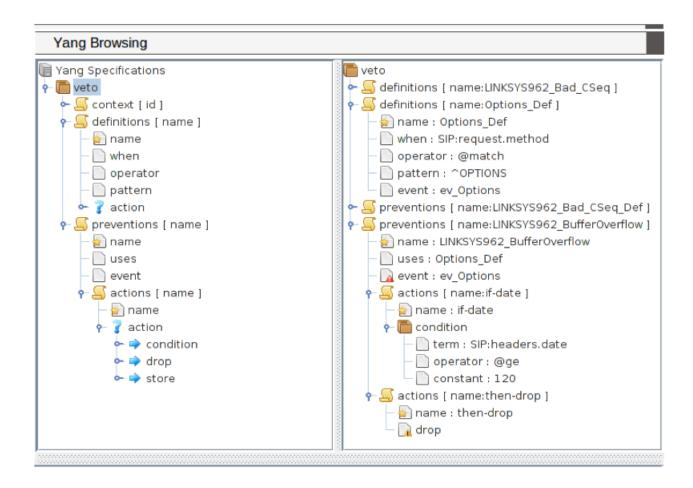
The YANG graphical user interface is implemented as a java applet running on the user manager station (User GUI in previous figure). The left part is the YANG data model and the right part is the YANG data tree of selected parts in the model.
