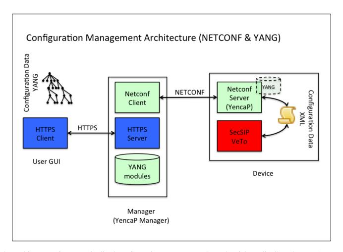
The architecture of our standardized configuration management is made of three distributed parts: the User GUI, the Manager and the Device. We use the IETF standardized approach to configuration management with the NETCONF [RFC4741] protocol and its data modeling language called YANG [YANG].
