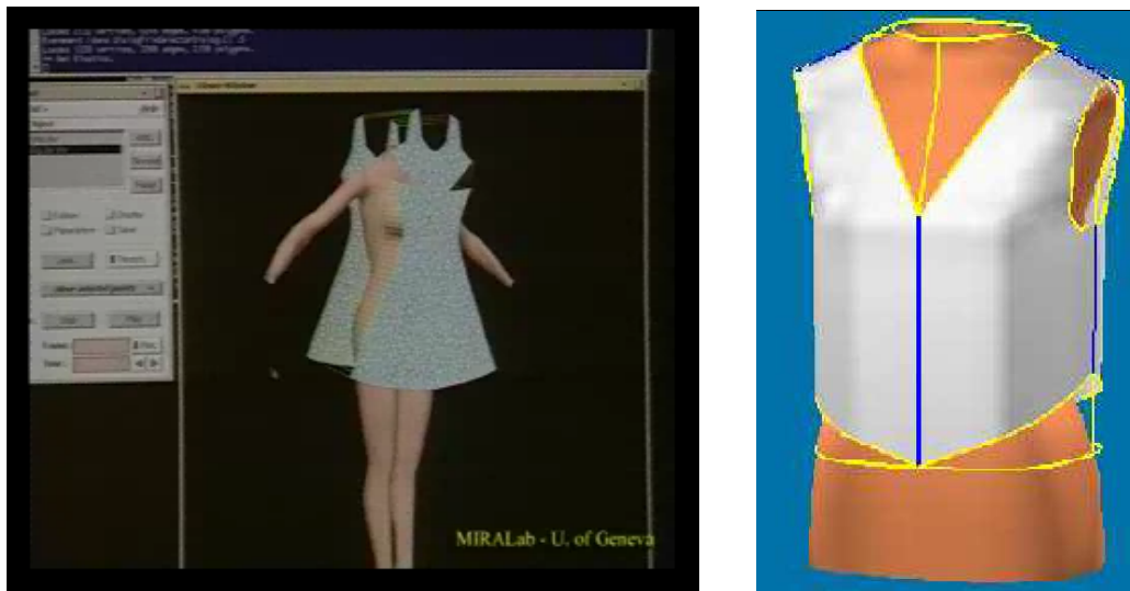
Figure 2.1: (left) Interface of the cloth design system from the Miralab. The user has drawn patterns in 2D and must place and seam them around a virtual mannequin, before launching a physical simulation. (right) Editable 3D cloth template, as described in [1]. The user modifies parametric curves standing for borders, seamlines, holes, darts...
