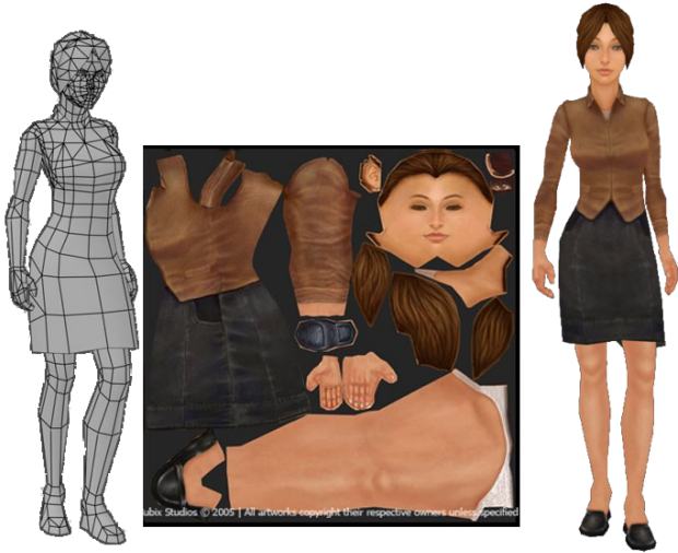
Figure 2: A low-polygon mesh and the associated texture (from Cubix studios), that was painted in 2D. Note how important parts (legs, hands, face) are kept. Note also that the legs (and also the two arms) are mapped to a single image, thus reducing texture storage.
