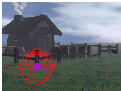
Figure 4 - “Virtual surround”. A virtual set of speakers (here located at the vertices of an icosahedron surrounding the listener) are used to spatialize any number of sources using 18 3D audio channels.
