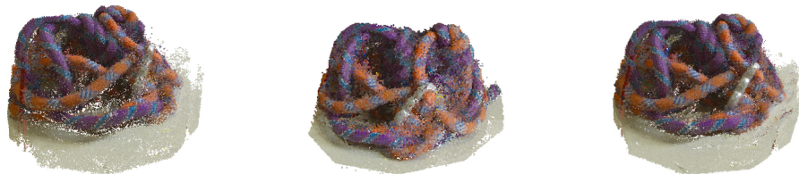
D: Comparing results with voxel coloring [23]. (left) 305,393 points randomly generated in 4 hours; (center) 200,968 points interactively generated in 45 min; (right) 517,307 points generated by our implementation of voxel coloring in 10 min.
