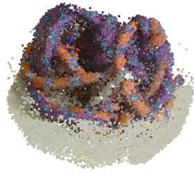
e) After depth map computation for each image, more points are generated in interior regions of the object (10s), improving color matching (total 45,000 points)
