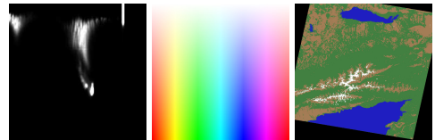
Figure 7: The hue-saturation histogram of the satellite image (which special treatment of gray colors) and the respective color table. The right image shows the classification of surface types for four clusters: water (blue), vegetation (green), rock (brown) and snow (white).
