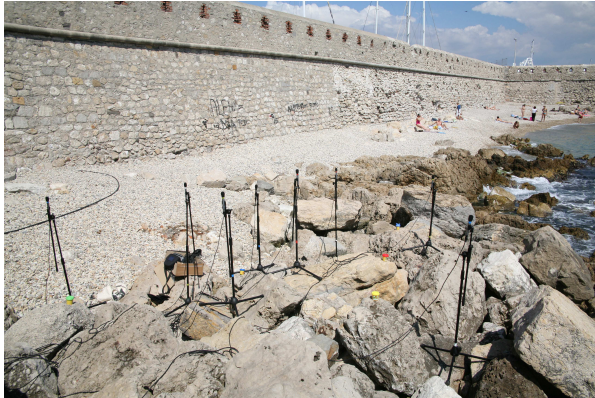
Fig. 9: Recording setup used for the seashore recordings.
