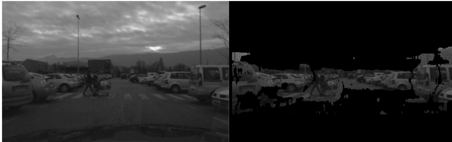
Figure 2: Depth mask example. The mask filters out the road surface and the objects that are over a prespecified height.
