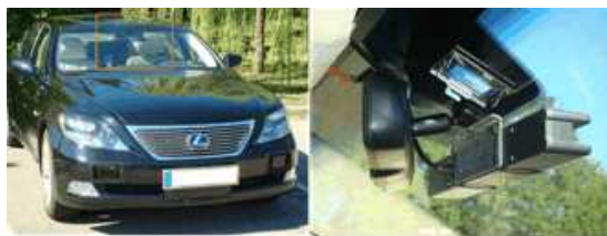
Figure 5: Our Experimental Platform. Lexus LS600h vehicle equipped with a TYZX stereo camera placed behind the windshield.
