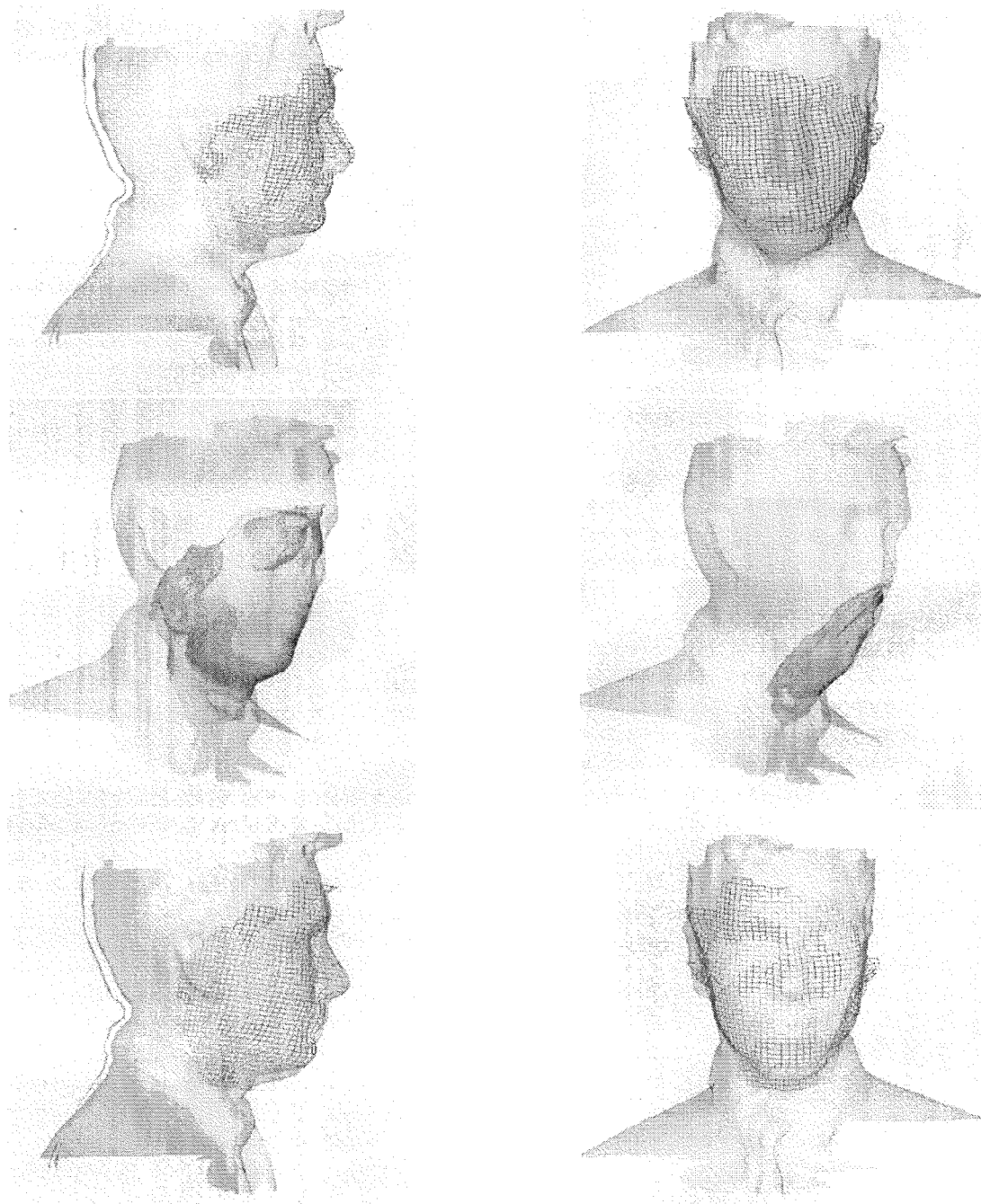
Figure 5. Top: The best rigid displacement found between the two faces. One surface is transparent, the other is represented by lines. When the lines are dark, they are in front of the transparent surface, when they are not, they are behind. Middle: Affine least square matching without additional constraints: The two surfaces after 45 iterations (left) and 75 iterations (right). The transformed surface tends to shrink and becomes very small. Bottom: The final affine transformation between the two faces. One can see, especially in the left images, that the nose, the mouth and the chin are now much closer. Quantitatively, the average distance decreases from 0.0193u to 0.0152u (the largest surface diameter is the unit), i.e., a 22% improvement for the affine transformation with respect to the rigid displacement.
