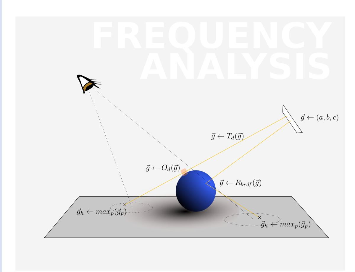
Durand et al. [2005] presents a Fourier analysis of the light transport in 4D. For efficiency reasons, we assume the radiance function to be isotropic in space and isotropic in angle, reducing the dimensionality of the spectrum of the radiance function to 2. We further approximate the spectrum by a gaussian:
