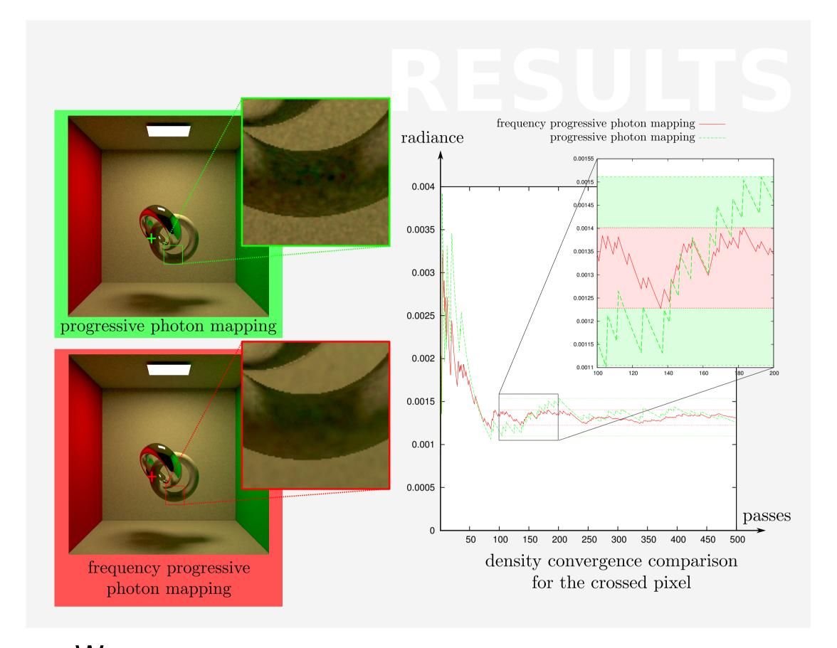
We update PPM by adding a frequency analysis step where the collected frequency photons' parameters will drive the radius reduction. We make the hitpoint's radius converge to a minimum radius defined as "bias free" (up to a user defined percentage) predicted by our frequency analysis. This allows to gather more photons per hitpoint when the minimum radius is reached and thus to reduce the variance of the estimate while avoid bias.
