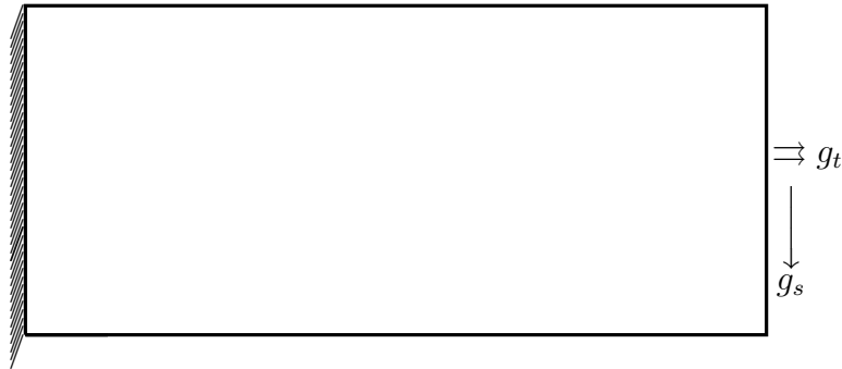
Figure 18: Boundary conditions: multiple loads case
