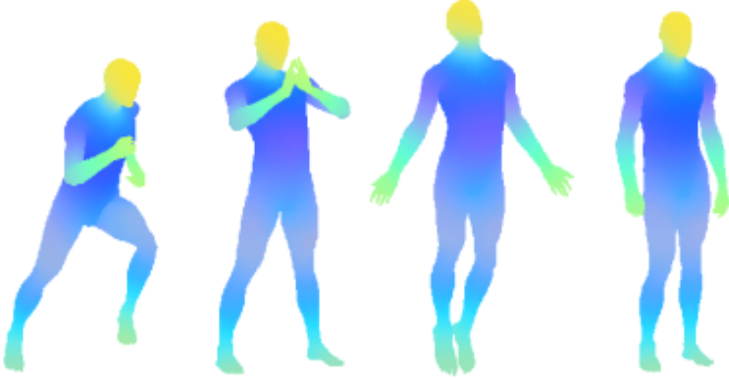
Figure 5: Invariance of the first three components of the HKS (shown as R, G, and B channels, respectively), for a shape undergoing isometric transformations.
