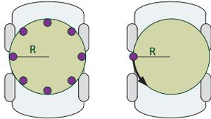
Fig. 2. Possible sensor deployment over a robot. Left figure:  $N$  sensors are fixed along a circular path at the top of the robot, with equispaced angles; right figure: a single sensor is rotating fast on the top of the robot.
