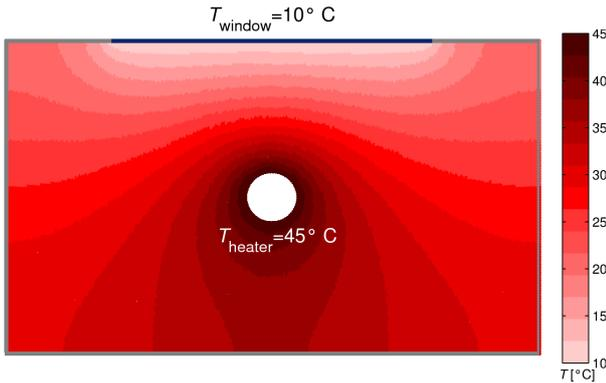
Fig. 1. Steady-state temperature in the room from Example 2
