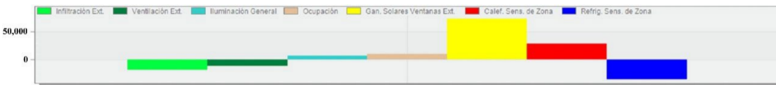
Figure 23. Analysis of energy gains and losses in the modified house using the software “Design Builder” (yellow column: solar gains of glass).
