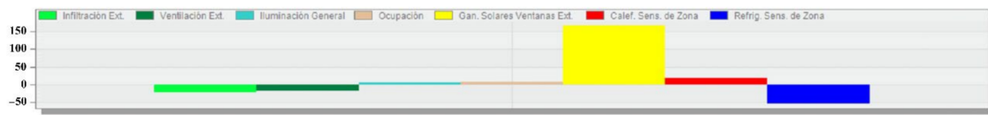
Figure 16. Analysis of energy gains and losses in the original house using the software “Design Builder” (yellow column: solar gains of glass).
