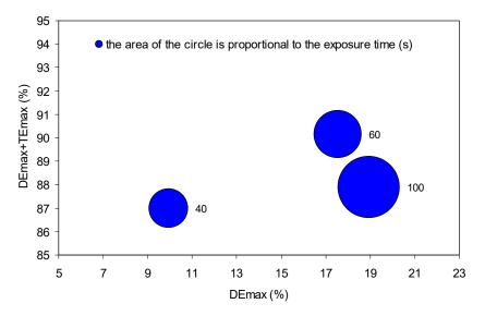
Figure 4. DEmax + TEmax versus DEmax for different exposure times during the hologram recording.
