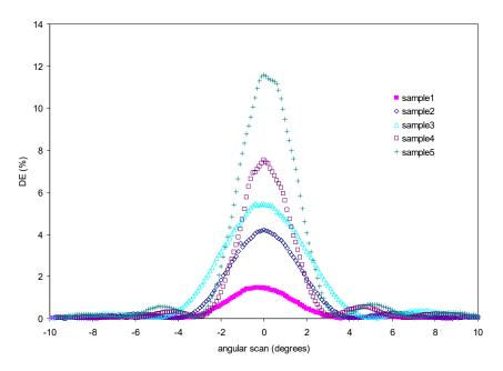
angular response curves obtained by the samples after the holographic recording and white light exposure.
