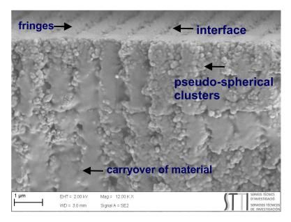
**Figure 8.** Enlargement of Figure 7 right showing aspects of the structure: interface between fringes, pseudo-spherical clusters that form the fringes, and areas with the carryover of material.
