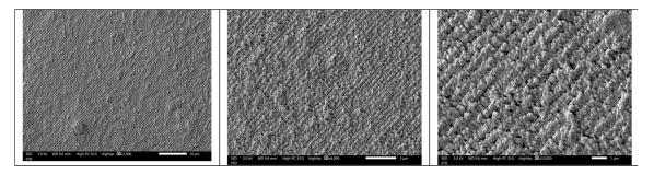
Figure 3. SEM images for a sample of HPDLC with peppermint oil (purity 80%).
