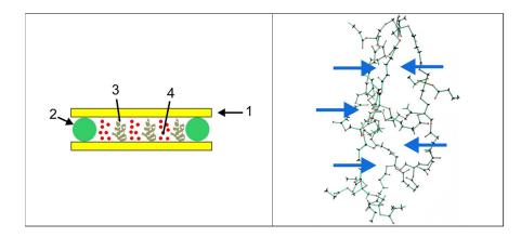
**Figure 2.** (Left) sample structure, 1: glass substrate, 2: microspacers, 3: exposed zones with polymer network, 4: unexposed zones with liquid crystal droplets. (**Right**) 3D polymer network from DPHPA. Arrows show holes in the network with a similar or higher size than an LC molecule.
