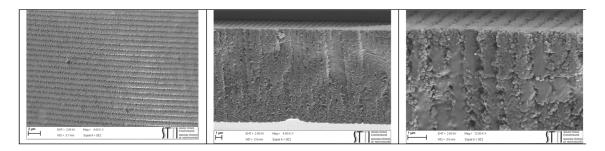
**Figure 7.** High-resolution SEM images for a sample of HPDLC with peppermint oil (purity 50%). Center and right images are taken by cross-sectional viewpoint.
