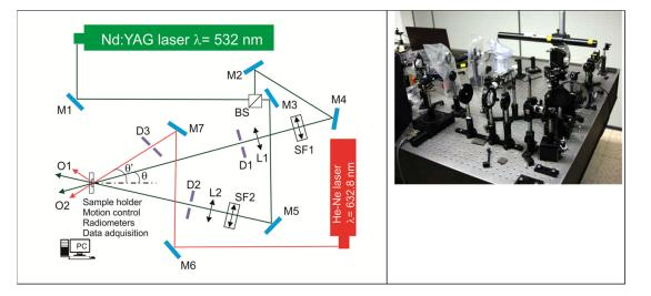
**Figure 1.** Holographic setup. BS: Beamsplitter, Mi: mirror, SFi: spatial filter, Li: lens, Di: diaphragm, Oi: radiometer, PC: data recorder.
