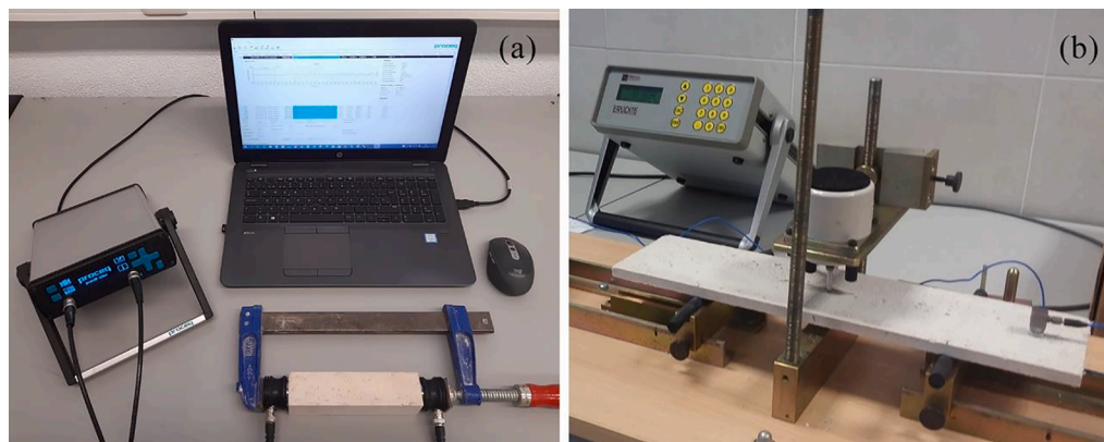
Fig. 4. Non-destructive tests set-ups: (a) measurement of ultrasonic wave propagation on mortar samples; (b) sonic resonance tests on TRM coupons.
