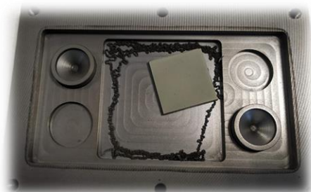
Figure 16: Kesterite just after being synthesized inside the graphite box. The residue surrounding it is the not consumed Sn.
