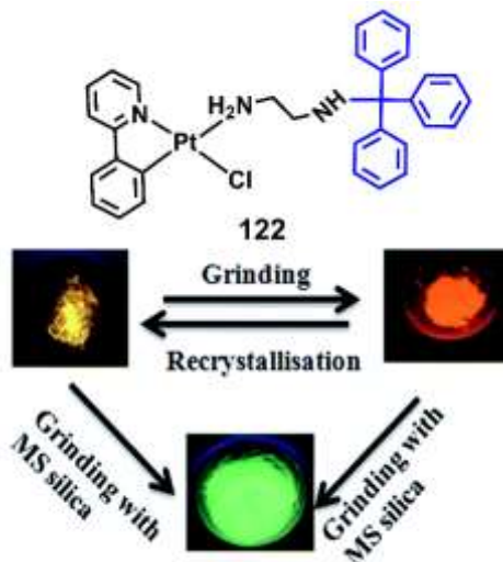
Fig. 32. Luminescent images of pristine complex 122 (yellow), 122 after grinding (orange), and after mixing 122 with mesoporous silica (photograph taken under 365 nm UV illumination). Adapted from ref. [181] with permission from The Royal Society of Chemistry.
