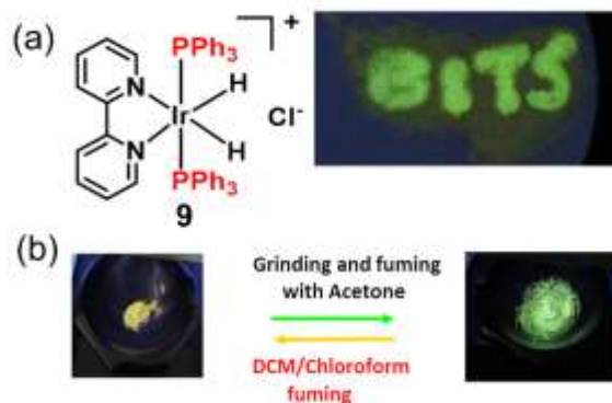
Fig. 26. (a) Molecular structure of complex of 9 (Cl - ) and picture of a filter paper coated with the complex where the word 'BITS' was written by using a capillary tube loaded with acetone, (b) Colour change of complex 9 (Cl - ) after mechanochromic and vapochromic response. Adapted from ref. [101] with permission from the American Chemical Society.
