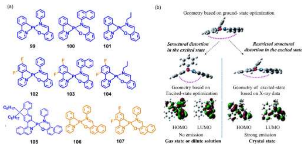
Fig. 24. (a) Molecular structure of complexes ( 99-105 ) (AIE-active) and ( 106, 107 ) (AIE-inactive), (b) Calculated geometries and molecular orbitals of complex 99 in different states. Adapted from ref. [174] with permission from The Royal Society of Chemistry.
