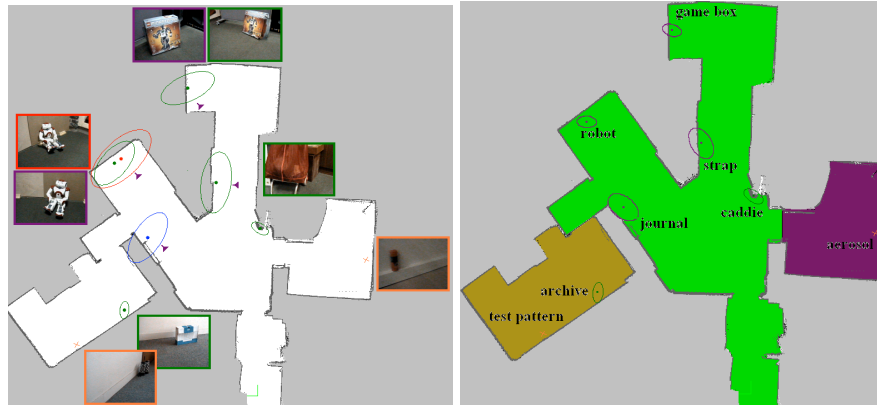
Fig. 5. Left: Semantic map showing the environment structure and the objects position with their ellipses of uncertainty. Right: Semantic map after the map improvement module.
