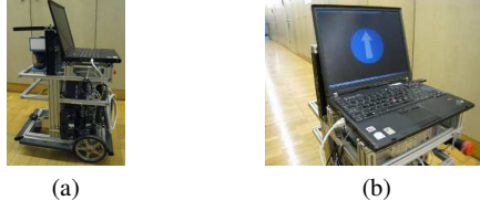
Fig. 2 (a) The differential drive robot used in our experiments. (b) Example of action proposed to the user, who then either agrees or disagrees orally (use of a speech recognition software).
