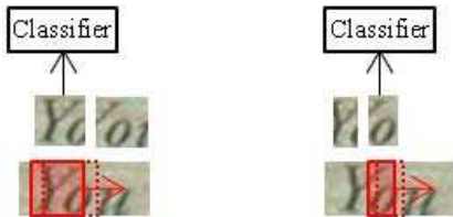
Figure 1. Multi-scale sliding window scheme: images on the left and on the right are respectively scanned with windows of sizes h and \frac{h}{2} and extracted sub-images correspond to windows placed at positions \frac{3h}{4} and h .
