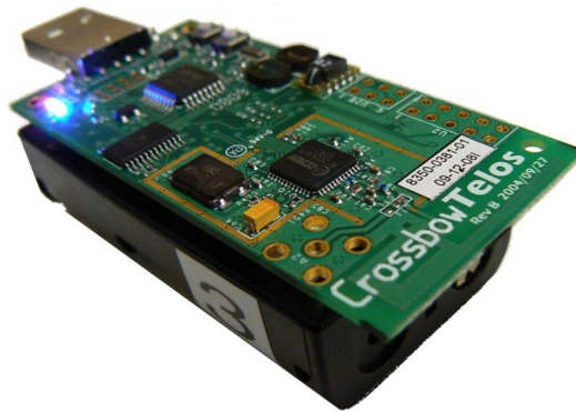
Figure 10: The TelosB mote.
