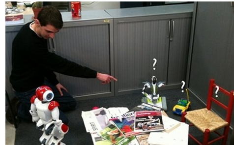
Fig. 2. To allow users to designate a particular object to a robot in a cluttered environment, we need to provide them with a robust and accurate pointing detection. Otherwise it may lead to restrictive interaction and even to false learning examples.
