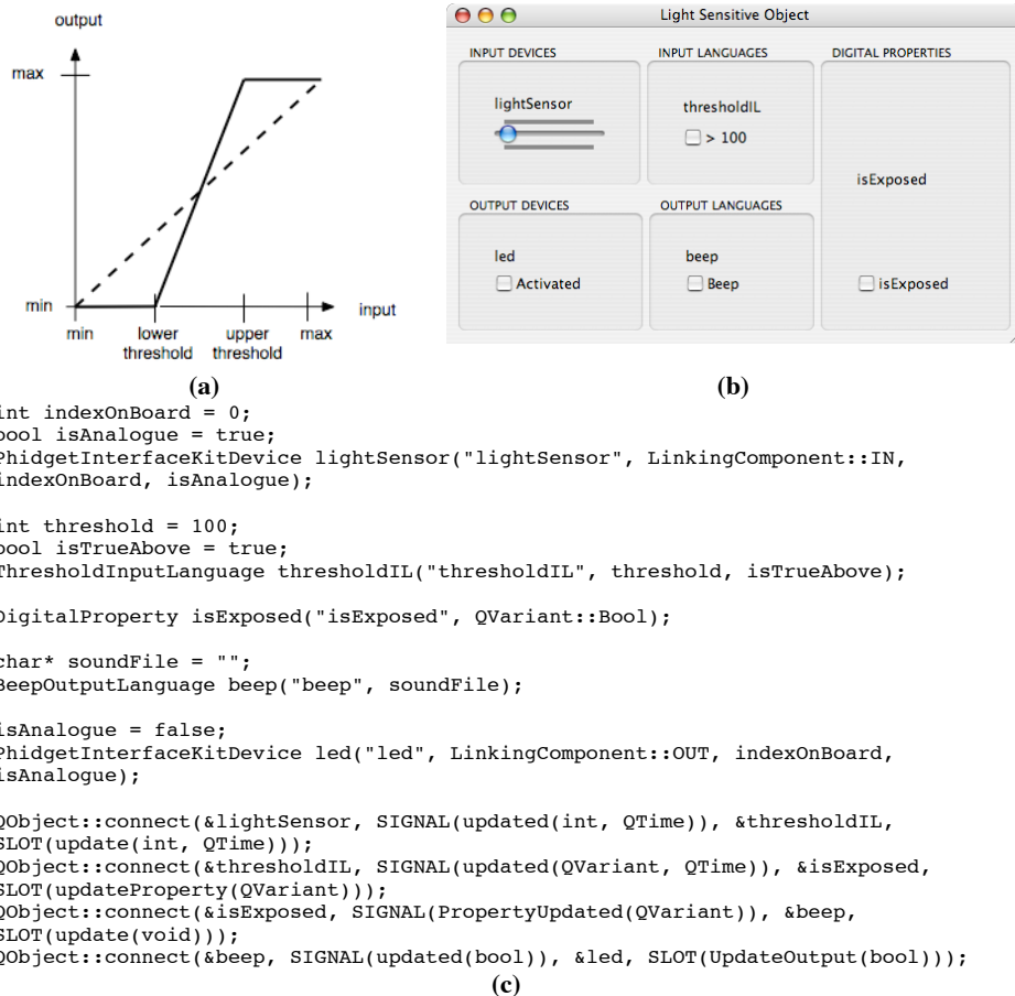
Fig. 5. (a) Two input linking language components: Identity (dashed line) and Ramp (plain line). (b) Graphical User Interface. (c) Code with inserted picture of a simple object built using OP.
