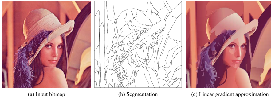
Fig. 6.10 The Ardeco system [17] converts an input bitmap into a collection of linear or radial gradients. The algorithm segments the image into regions well approximated by the elemental gradients. ©Copyright 2006 Eurographics.
