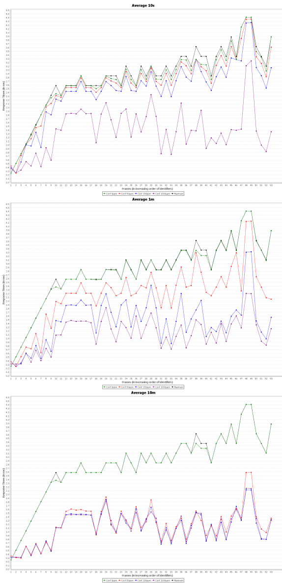
Figure 2: Simulation statistics with initial phasings leading to worst case response time for the frame 49. From top to bottom, the graphics show the frame response time for the first 10s, 1mn and 10mn of simulation. The X-axis are the frames sorted by decreasing order of priority. The black curve is the maximum response times recorded without drift. The other curves are the average response times recorded without drift (green) and drift bounds resp. equal to 50 ppm (red), 150ppm (blue), and 1000 ppm (purple).
