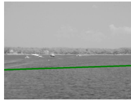
(a) Image processing on frame 47 without gyro tracking. A wave is detected as the horizon.
