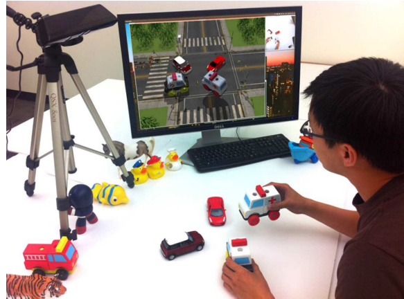
Figure 20: A system for producing 3D animations using physical objects (i.e., puppets) as input [HGCA12]
