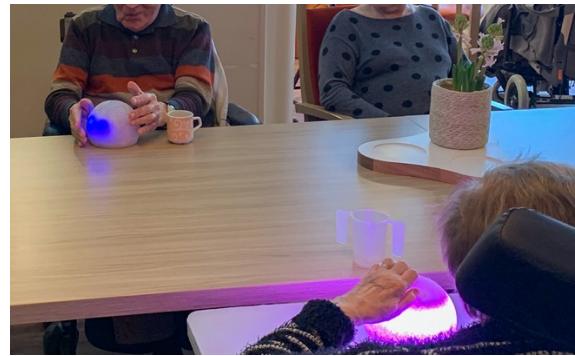
Figure 6: SAM offers multisensory stimuli, such as colored lights, sounds, and vibrations, to draw the attention of people with dementia.
