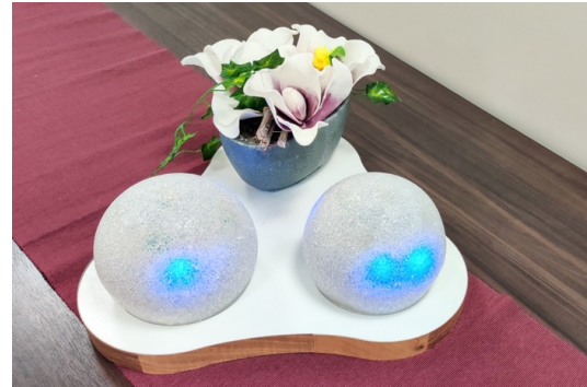
Figure 2: SAM is an interactive companion that plays sounds and displays colors in response to touch-based inputs and can mimic or react to the input of a paired device to stimulate social engagement between care home residents.
