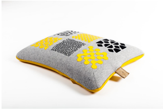
Figure 3: VITA is a cushion equipped with conductive textile sensors that offer a touch-based input for playing audio content.
