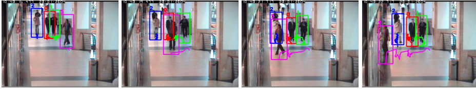
Fig. 4. Tracking results of four persons in the sequence ShopAssistant2cor (Caviar dataset) are correct, even when occlusions happen.
