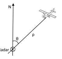
Figure 1: Positioning of the Aircraft in Relation to the ATC Radar
