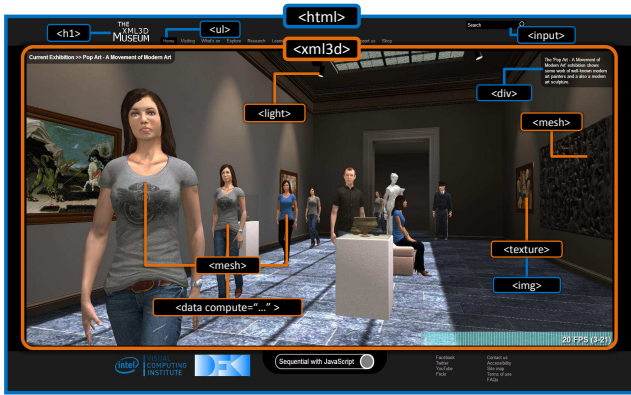
Figure 3: A highly dynamic declarative 3D scene with nine animated and skinned characters. The calculation is either performed with classical sequential JavaScript or in parallel exploiting Intel’s River Trail proposal for parallel data computations in JavaScript.
