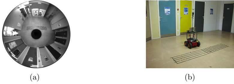
Figure 10: Desired position. (a) The omnidirectional image acquired at this position and (b) corresponding external view of the mobile robot.
