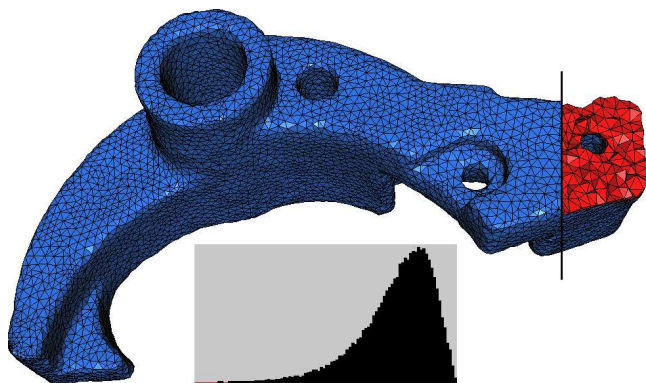
Figure 8 Mechanical model: 15,687 vertices and 71,757 tetrahedra.
