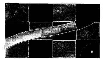
Figure 1: The application domain showing the subregions defined to (a) handle the singularity and boundary layer, (b) use 16 processors on the problem: 12 for Region A, 3 for Region C and 1 for Region B.
