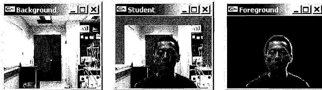
Figure 8. Frame, background, and video sprite compute by background subtraction.
