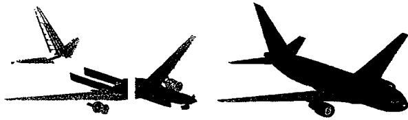
Figure 8. Layers of the aircraft finite element model.
