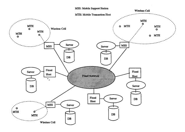
Figure 1: Mobile Database System Model
