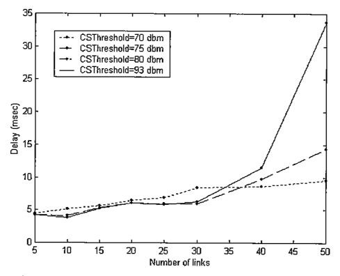
Transmission delay for different loads
