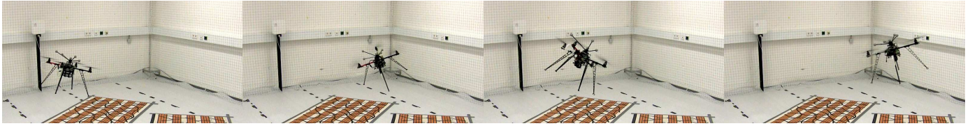
Fig. 5. Snapshots of the quadrotor executing an 8-shaped trajectory
