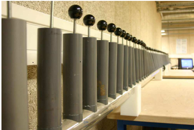
Figure 1: Tube connected with Helmholtz resonators (courtesy given by O. Richoux).
