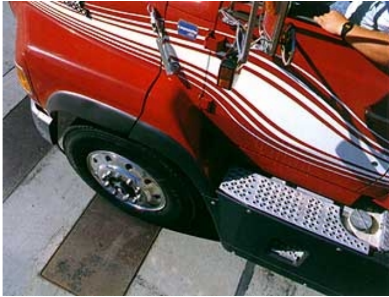
Figure 3-6: Front axle of truck passing over Bending Plate
