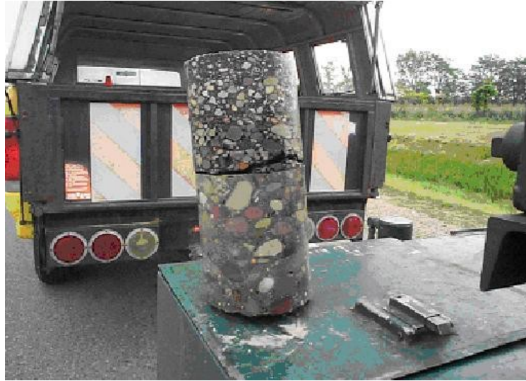
Figure 6-2 Core Sample of Composite Pavement
