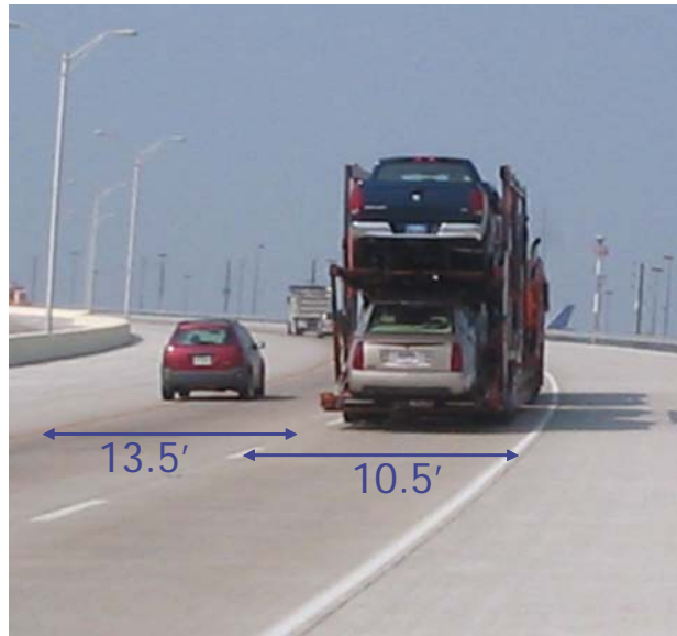
Figure 8.5 Constant lane width assumption proven false
