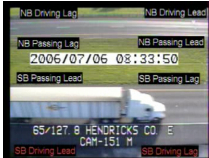
Figure 4.4 View from PTZ Camera showing Autoscope 2020 Overlay and Dynamic Label Detectors
