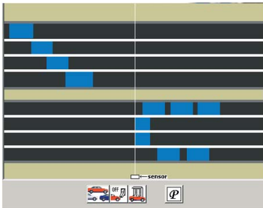
Figure 4.18 Example of Wavetronix SmartSensor Manager Lane Configuration GUI, showing four lanes in each direction of travel
