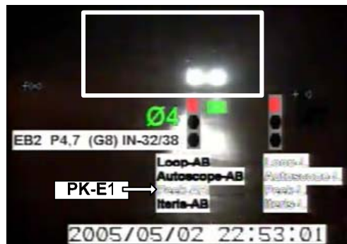
b) PK-E1: Vehicle in detection zone is dropped because headlights are past stop bar.
