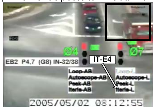
h) IT-E4: Large vehicle in Left-turn lane is beyond stop bar but still in video detection zones due to its' height.
