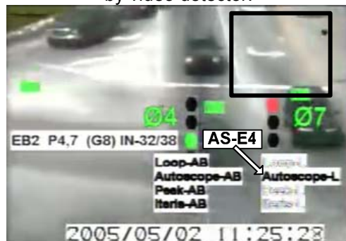
g) AS-E4: As vehicle creeps beyond stop-bar call is maintained.
