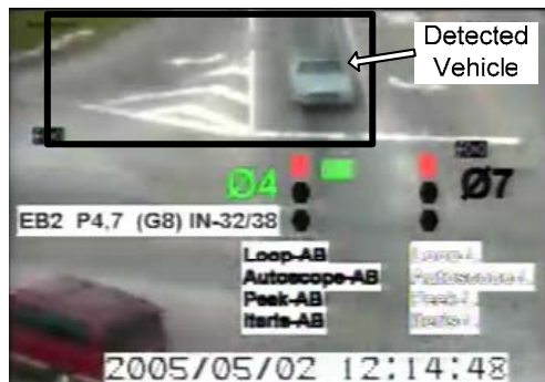
a) IT-E1: Vehicle in through lane is correctly detected.
